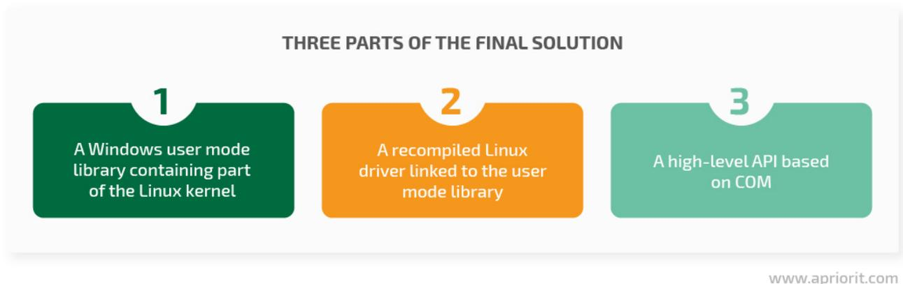
We combined the resulting components in a single Windows service. This service is responsible for detecting WiFi USB devices and switching their drivers between the standard drivers and our WinUSB driver.
